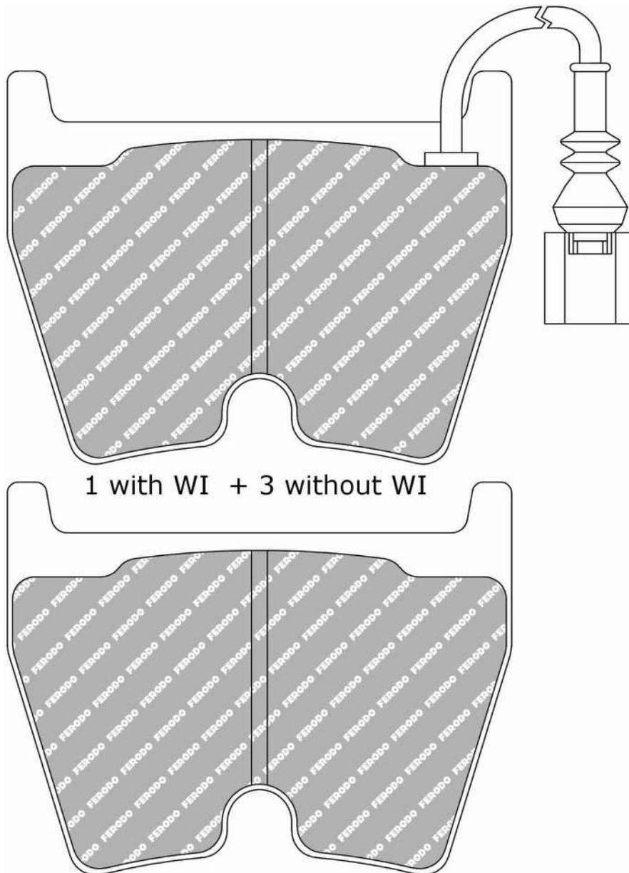
4 Piston caliper -> 1 axle = 2 sets (8 pads) Remove electronic wear indicator cable from set for vehicle's left hand caliper.
